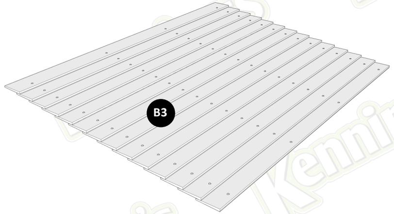
Remember to leave a 20mm overlap on each board and to screw through the thick part of the featheredge board.
